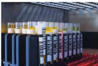
2D Barcode Reagent Identification
